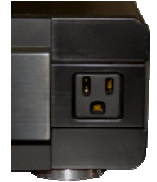
Front-mounted convenience outlet
